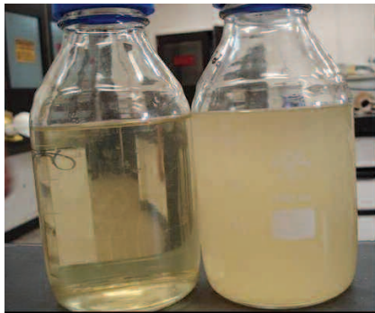
Condensate samples collected at Site C at the outlet (left) and inlet (right) of Pall's coalescer test unit
