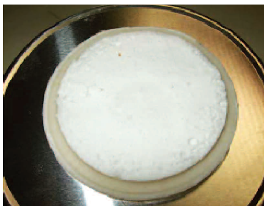
Figure 6: Filter cake shown collecting on the T2100 media
