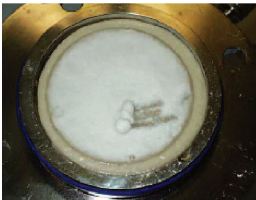
Figure 5: Filter cake shown collecting on the T1000 media
