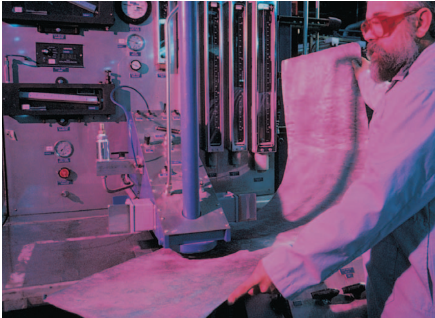
Bubble Point Testing Metallic Media
