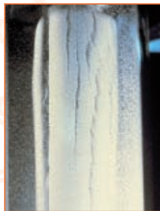
Reverse flow effectively dislodges nonpermanent cake.
