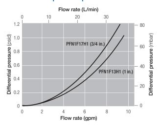
$^{5}$  For liquids other than water, multiply the pressure drop by the specific gravity of the fluid.
