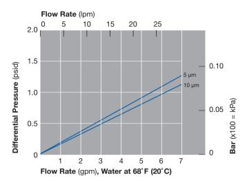
Flow rate is per 10" (25.4 cm) element. For liquids other than water, multiply differential pressure by fluid viscosity (cP).
