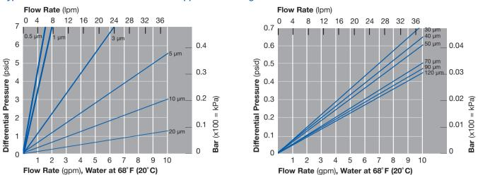
Flow rate is per 10" (25.4 cm) element. For liquids other than water, multiply differential pressure by fluid viscosity (cP).
