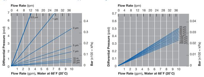
Flow rate is per 10" (25.4 cm) element. For liquids other than water, multiply differential pressure by fluid viscosity (cP). Due to the very low flow resistance of the media in the more open grades, pressure drop is primarily related to turbulent loss through the center core.
