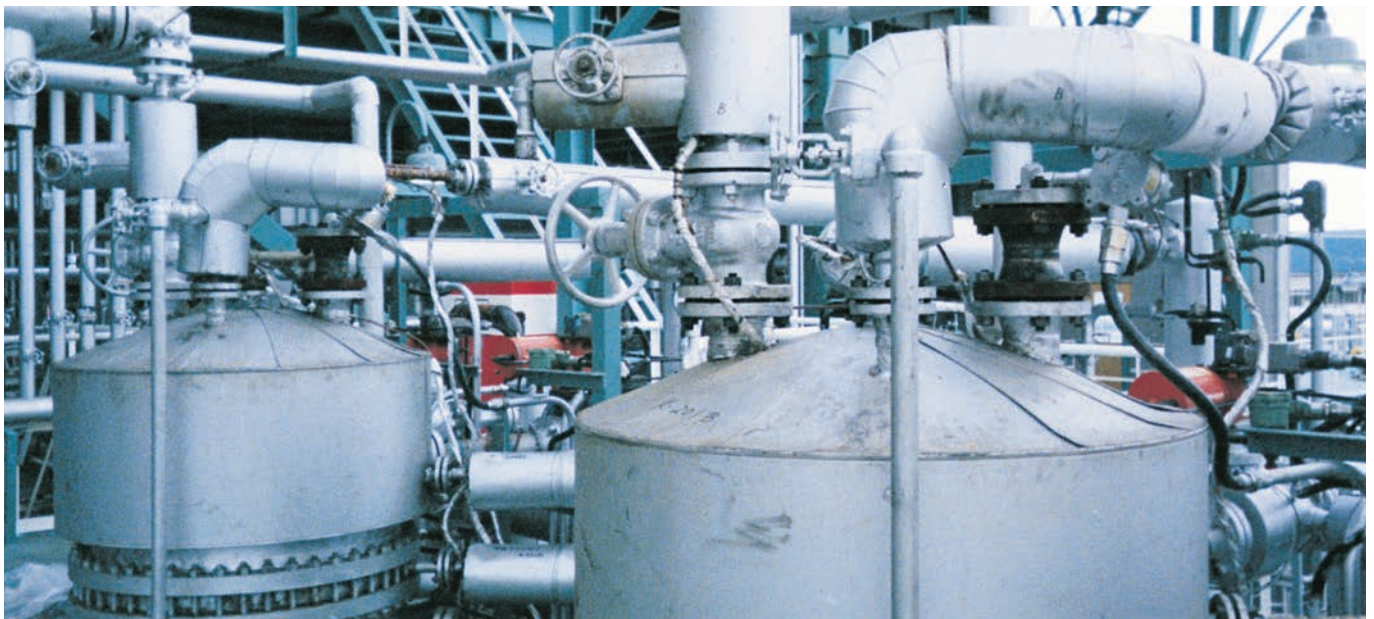
Pall's blowback filters are used to remove catalyst fines from vent gas.
