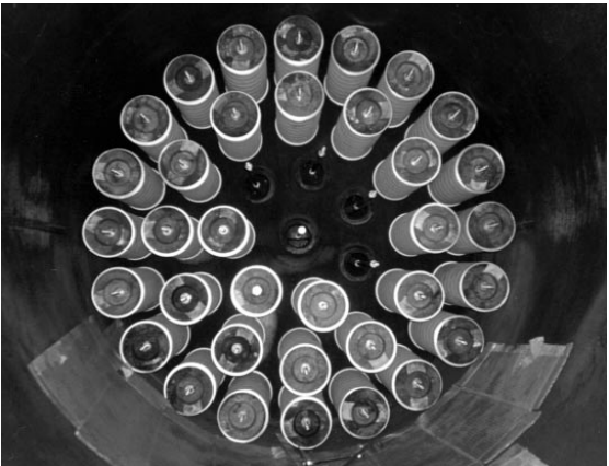
Figure 3: Installation of Pall PhaseSep FR1 Coalescers onto Pall Retrofit Tie-Rods.
