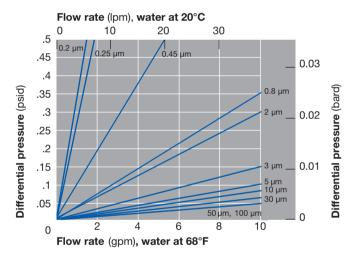
Flow rate is for a 25.4 cm (10 in) cartridge. For liquids other than water, multiply differential pressure by fluid viscosity (cP).
