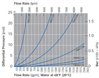
To calculate the actual housing pressure drop, multiply this aqueous pressure drop by the fluid's specific gravity. This value must be added to the filter pressure drop to calculate the overall pressure drop of the filter system.
