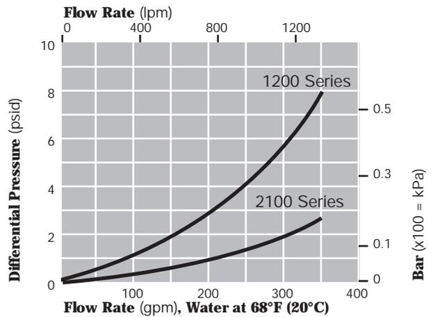
*For liquids other than water, multiply differential pressure by specific gravity.*
