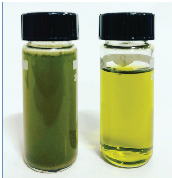
Figure 7: Cannabis oil samples from an ethanol extraction process. Raw oil (left), after filtration with SUPRA technology for clarification (right).
