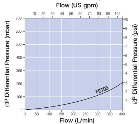
\* The flow/pressure drop curve refers to the empty housing only, for water at 20 °C (68 °F). For other liquids, multiply housing pressure drop by the specific gravity of the fluid.
