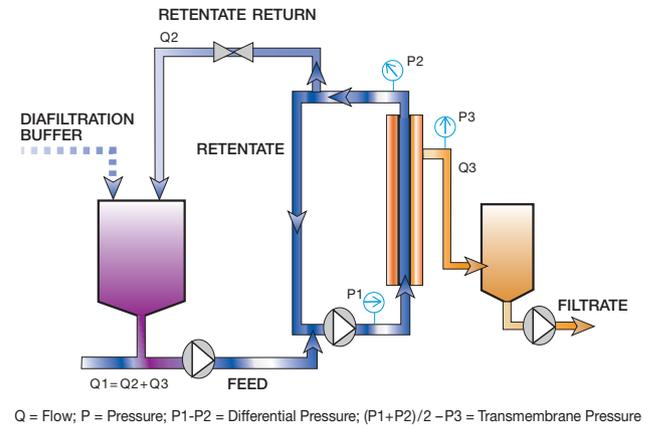
Examples of crossflow filters typically used in the food and beverage industry are the widely available systems using longitudinal modules consisting of polymeric (e.g. hollow fibers, spiral wounds) or inorganic (e.g. ceramic, sintered metal) membrane materials (Figures 8a–8b).
