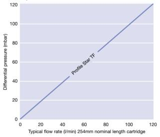
Note: Differential pressures are for liquids with a viscosity of 1 centipoise (cP). For cartridges of 508mm, 762mm, 1016mm nominal length, divide the differential pressure by 2, 3 and 4 respectively. To obtain the total pressure drop of a complete filter assembly the housing pressure drop must be added. Please refer to the relevant housing literature or contact Pall.
