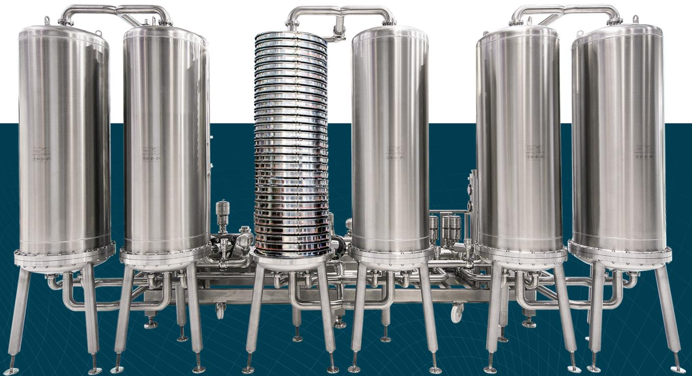
Pall's CBS System combines approved materials in beer stabilization (PVPP) with a new technology, enabling continuous stabilization of all types of beer. This streamlined process also enhances product consistency and maximizes throughput at volumes ranging from 80 hl/h to 800 hl/h. The system can be easily integrated with continuously operating membrane filtration systems and allows flexible handling of varying stabilization demands for different types of beer.
