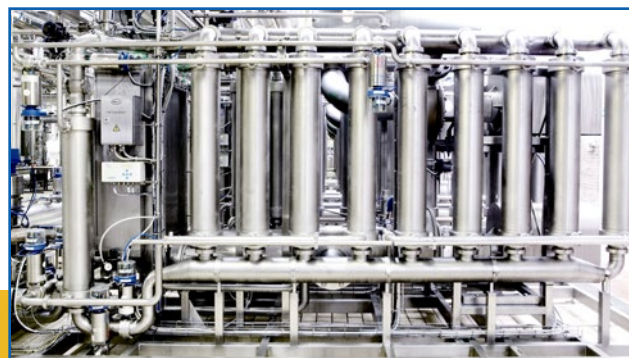
Typical filter block with 20 membrane inserts split in 4 clusters and a lowered modules
