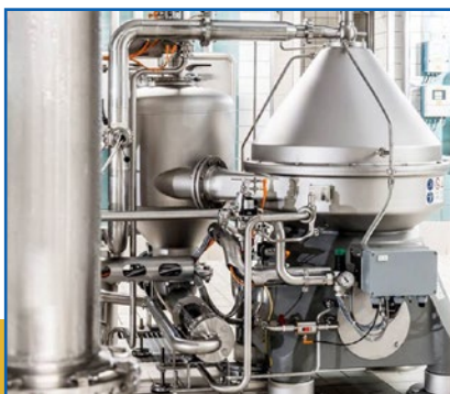
Typical centrifuge for pre clarification upstream filtration for 400 hl/h performance
