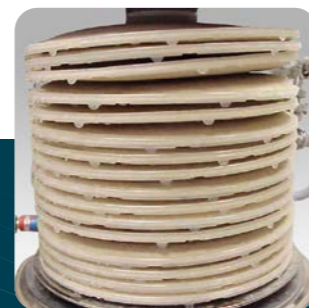
Figure 4: Cell deformities after heat treatment
