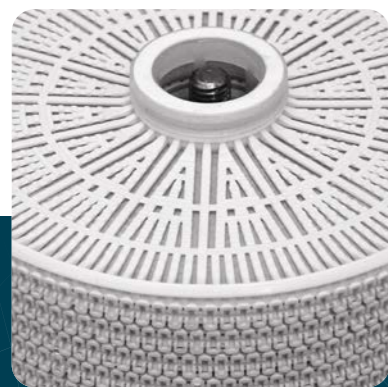
Figure 9: No damage to the SUPRAdisc II modules
