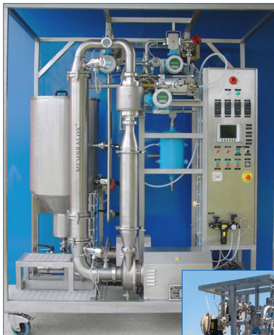
Examples of highly instrumented semi-automatic Membralox pilot unit available for rent
