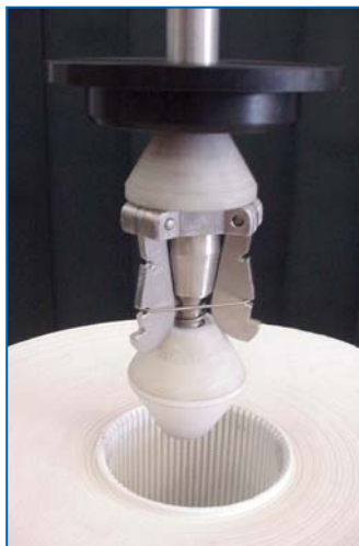
Figure 4: Hooks grab the bottom of the SUPRApak module stack for easy handling.
