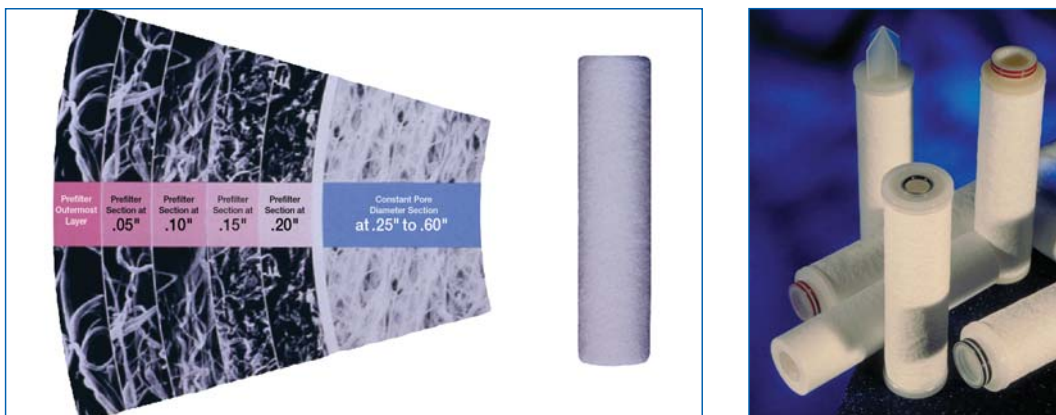
Figure 6: Profile II and Nexis® T cartridges are ideally suited for clarification due to their graded pore structure.
