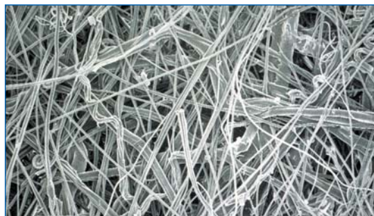
Figure 1a: SEM image of fibrous media
