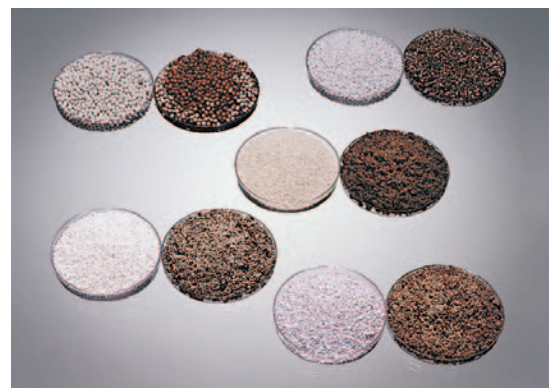
Left: Clean desiccant. Right: Fouled desiccant. Change-out and regeneration cycles will be significantly extended using Pall's SepraSol liquid/gas coalescers.
