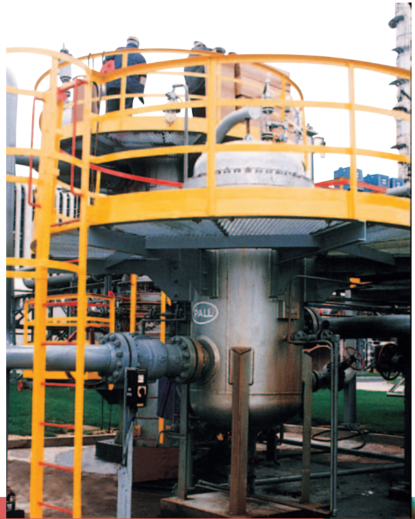
Vertical AquaSep Plus liquid/liquid coalescer system removing water from diesel.
