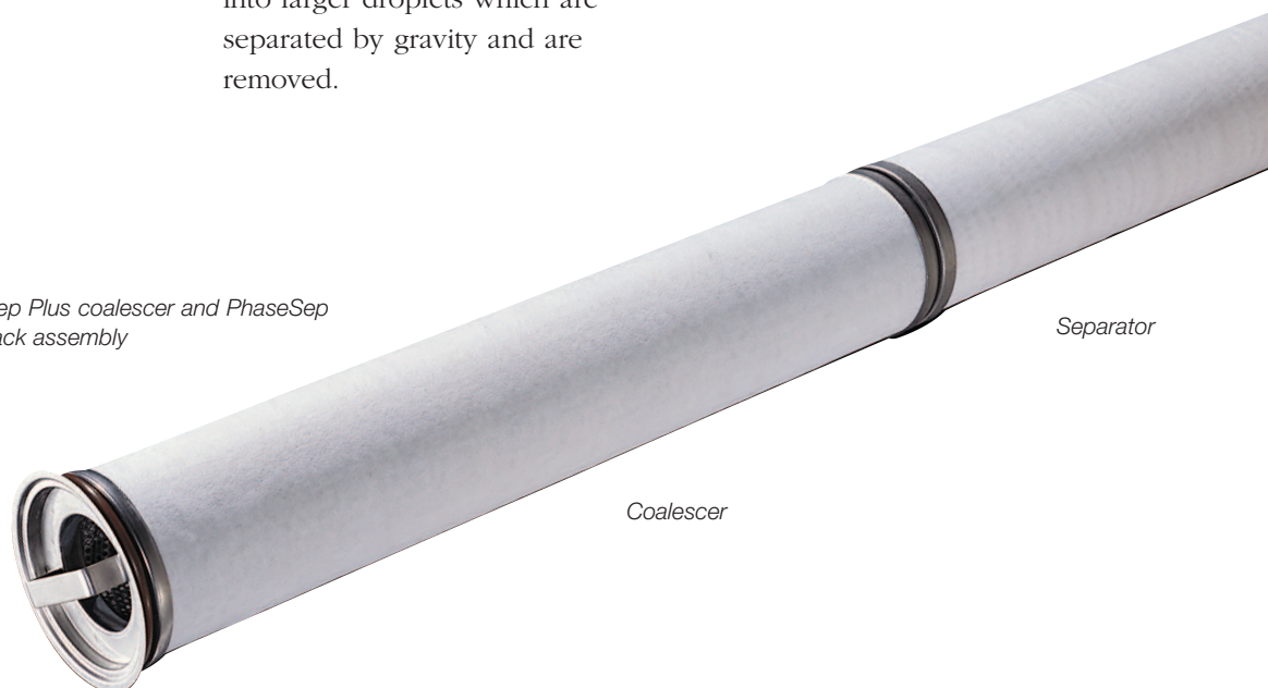
Pall horizontal liquid/liquid coalescer Configuration with prefilter far left and AquaSep Plus/PhaseSep coalescer shown right. Contaminant-free continuous phase exits top right, liquid contaminant exits bottom right.
