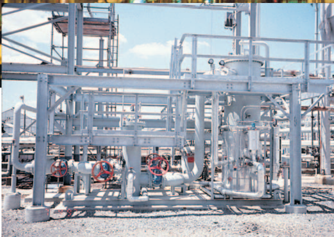
Vertical AquaSep Plus liquid/liquid coalescer system removing water from jet fuel.
