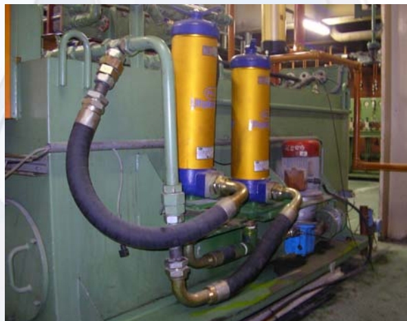
Pall Ultiplex SRT UR619 Series filters on off-line loop circuit
