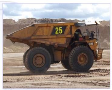
218 Tonne Payload Haul Truck
