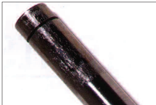
Figure 1: Injector plunger showing abrasive wear.
