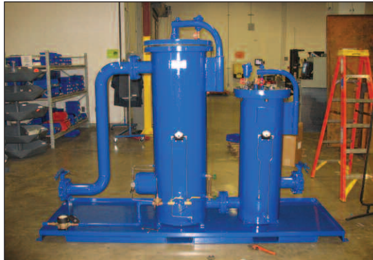
Figure 3: Typical filter and coalescer system utilized in mining operations capable of 300 GPM.
