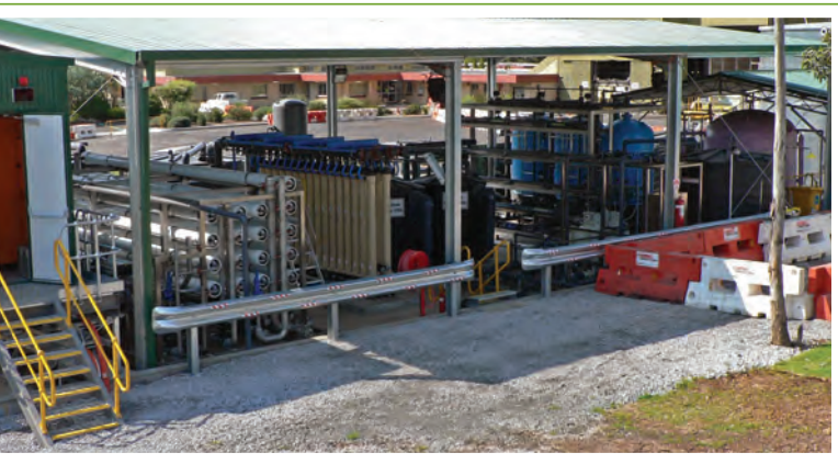
Recycling of treated mine drainage/discharge water for process and potable purpose within coal mining industry, Australia
