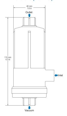
For best performance module should be Installed vertically. For best performance module, ink should be Introduced Into the module slowly to eliminate any possibility of air being trapped in the module.
