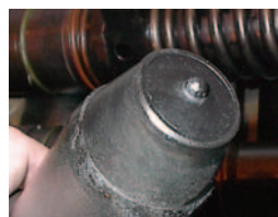
Large Diesel Engine Fuel injector with blocked injector nozzels caused by fuel contamination
