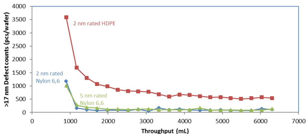
Figure 4. Defect counts > 17 nm threshold on bare Si wafer vs. throughput of POU filtration right after filter installation in CLEANTRACK LITHIUS Pro-Z. Test fluid was TOK OK73 thinner. Test filter format is Pall PhotoKleen EZD-3XL. Defect inspection was conducted using KLA-Tencor Surfscan SP5<sup>XP</sup>.
