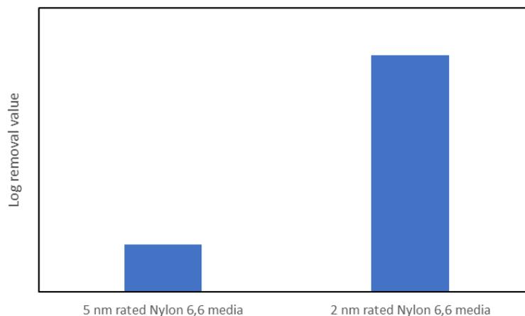
Figure 2. 2 nm gold nanoparticle retention of 2 nm and 5 nm rated Nylon 6,6 filters. Gold nanoparticle challenge test in DI water. Log removal value= $\log_{10}$ (particles in upstream side of the filter divided by particles in downstream side of the filter).
