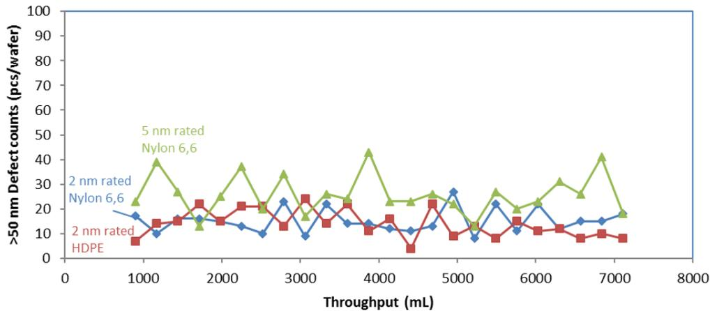
Figure 5. Defect counts > 50 nm threshold on Si wafer vs. throughput of POU filtration after replacing the pre-wet solvent with photoresist. Test fluid was TOK positive tone ArF immersion resist. Test filter format is Pall PhotoKleen EZD-3XL. Defect inspection was conducted using KLA-Tencor Surfscan SP5<sup>XP</sup>.
