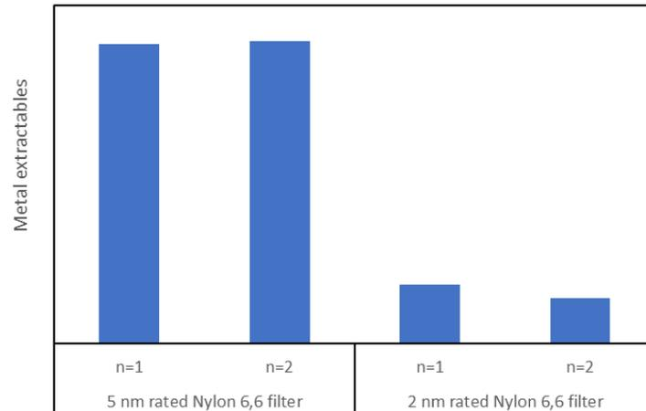
Figure 3. Total metal extractables (Li, Na, Mg, Al, K, Ca, Ti, V, Cr, Mn, Fe, Co, Ni, Cu, Zn, As, Ag, Cd, Sn, Ba, W and Pb) in DI water for PhotoKleen EZD-3XL filter with Nylon 6,6 media. Soaking duration is 24 hours.
