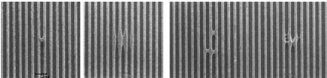
Figure 6. Bridge defect SEM images in after development inspection. 40 nm half pitch L/S fabricated with positive tone ArF immersion process.
