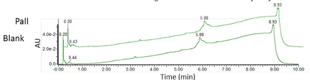
As shown in Figure 2, the Pall Acrodisc syringe filter with PTFE membrane provides a clean chromatogram following extraction with acetonitrile. By having little to no effect on the sample, the analyst can be confident that the data generated is accurate and has not been compromised by the presence of unwanted chemicals.
