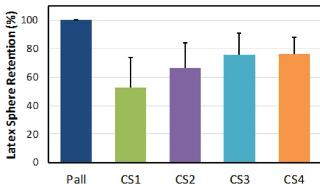
Figure 1 shows the latex sphere retention of syringe filters with pore size ratings of 0.2  $\mu\text{m}$ . The data shows that the Pall PTFE syringe filters (Pall) have higher retention efficiencies than other commercial syringe filters with PTFE membranes (CS1-4).
