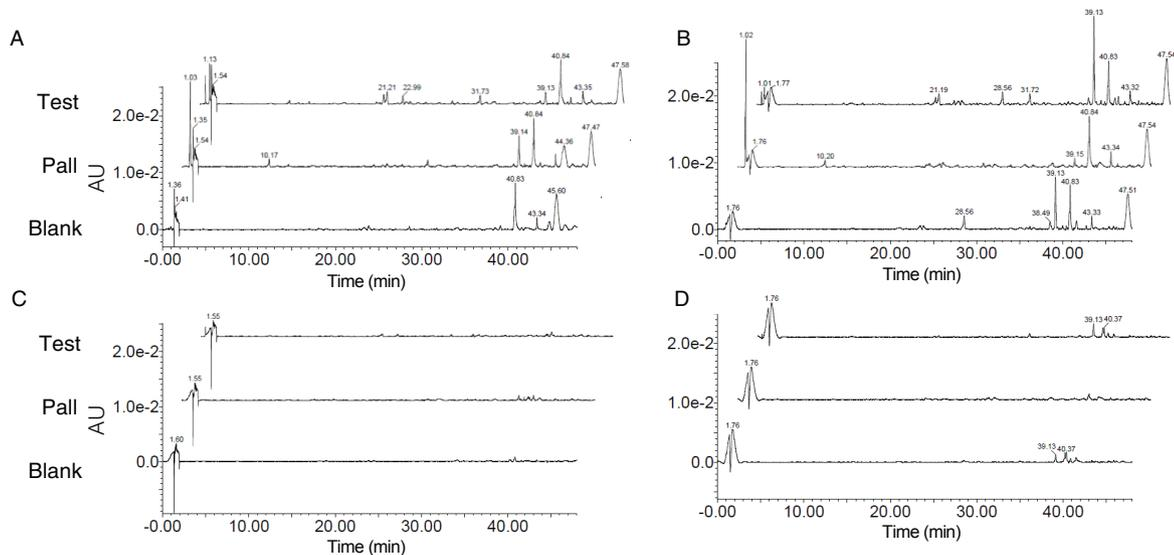
As shown in the data presented, the universal nature of the wwPTFE membrane can provide cleaner chromatograms than the regenerated cellulose filters in multiple solvents and across multiple wavelengths. By having little to no effect on the sample, the analyst can be confident that the data generated is accurate and has not been contaminated by the presence of unwanted chemicals.
