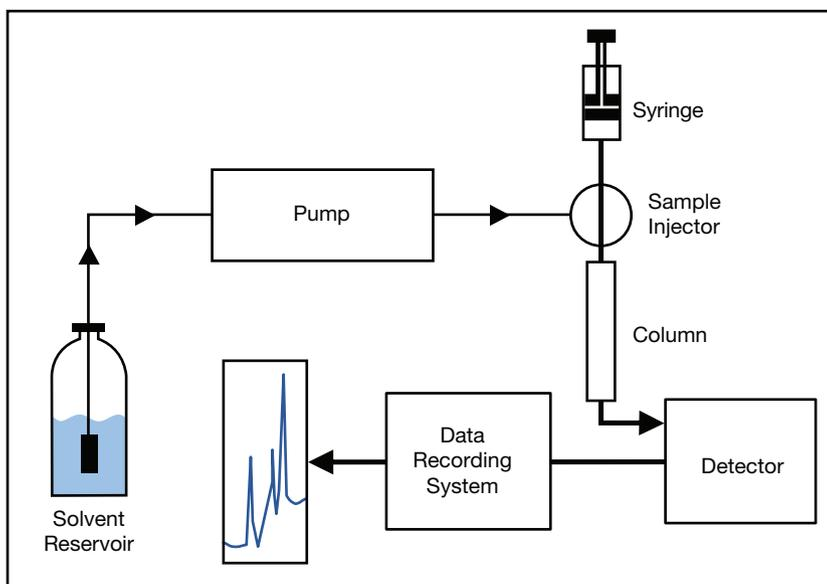
*Of the four common causes for HPLC column failure – plugging, voids, absorbed sample and chemical attack – plugging is the most frequently encountered by analytical chemists or analysts. Injection of samples containing particulates will eventually block the column inlet and column packing, cause high column back-pressure and shorten the normal lifetime of the column.*
