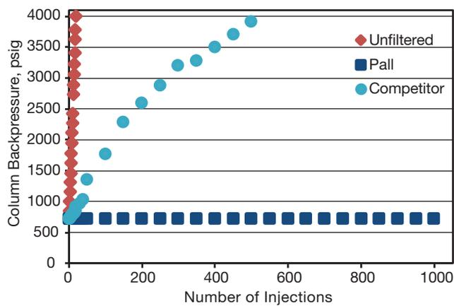
In the Analytical Technical Guide, we have shown that particulate removal through filtration can extend column life up to at least 52 times (Figure 2) over unfiltered samples. In addition to extending the life of the column, particulate removal also protects the pump, injector, and other components from premature wear.
