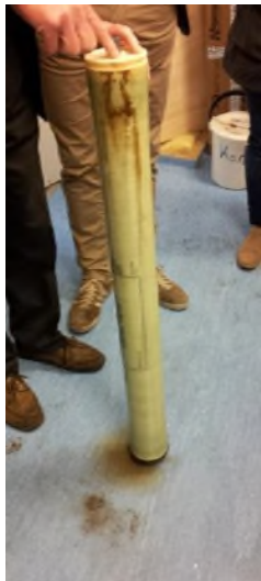
Blocked RO membrane due to inorganic and biological fouling
