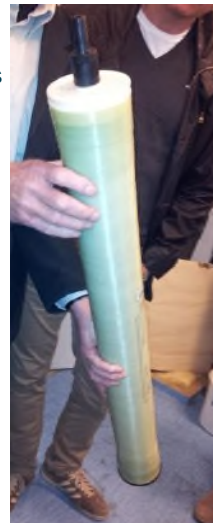
Clean RO element after Pall MF-Pre-treatment
