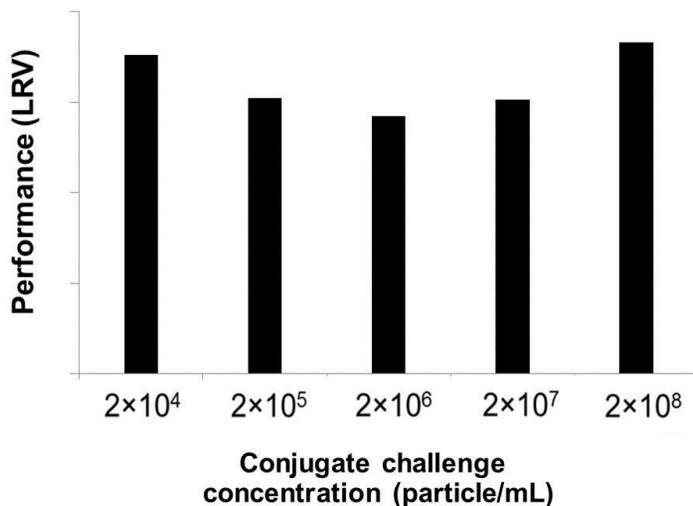
Figure 6. Dendrimer retention performance of 10 nm pore-rated nylon filter membrane with different challenge concentrations of conjugate. Nylon membrane performance is independent on dendrimer challenge concentration. Standard deviation of the LRVs is within the 10% of the mean LRV of all the tests.
