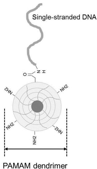
Figure 1. Schematic of a 5.4 nm DNA-dendrimer conjugate. A single stranded DNA chain (66 bases) is attached to the amino functionalized PAMAM dendrimer by an amide bond for producing a stable conjugate.
