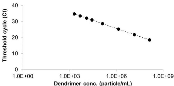
Figure 2. Dynamic range and sensitivity of detection of dendrimer by qPCR. Inverse relationship between qPCR threshold cycle with dendrimer concentration. This new method can detect and quantify 5 nm dendrimer particles up to a concentration of 2000 p/mL.
