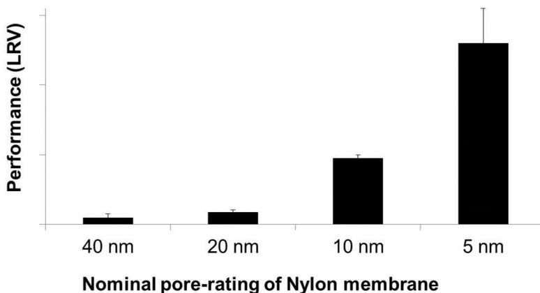
Figure 4. Dendrimer retention performance of various nominal pore-rated nylon filter membranes. Error bar is standard deviation of triplicate measurement. Conjugate test is capable of discriminating various nominal pore-rated nylon filter membranes.
