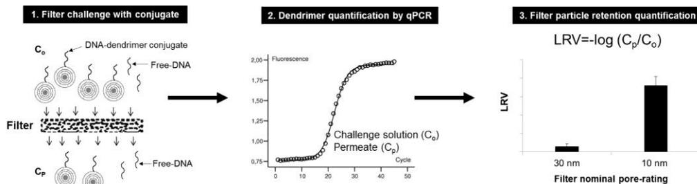
Figure 3. Schematic of DNA-dendrimer conjugate testing method. Testing is performed in 3 steps including, filter membrane challenge, dendrimer quantification by qPCR, and dendrimer retention performance quantification of filter membrane.
