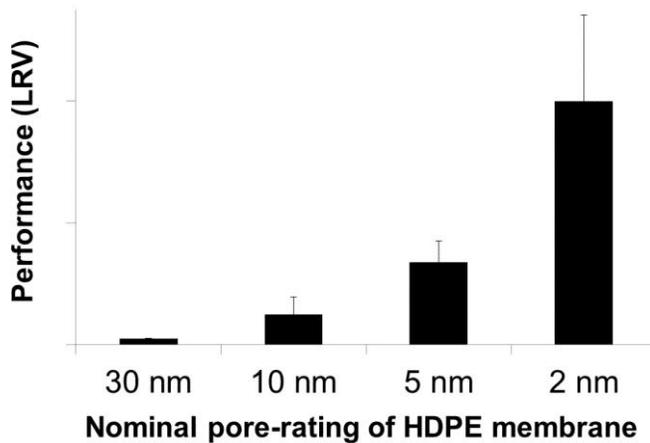
Figure 5. Dendrimer retention performance of various nominal pore-rated HDPE filter membranes. Error bar is standard deviation of triplicate measurement. Conjugate test is capable of discriminating various nominal pore-rated HDPE filter membranes.
