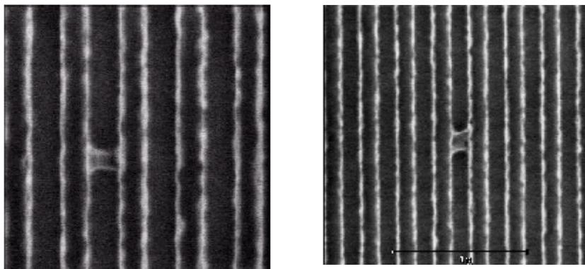
Figure 1: Typical trench bridging defect<sup>1</sup>
