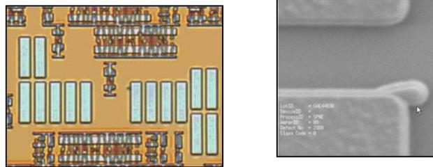
Fig.6: Typical poly blocked etch defects (optical and SEM image)
