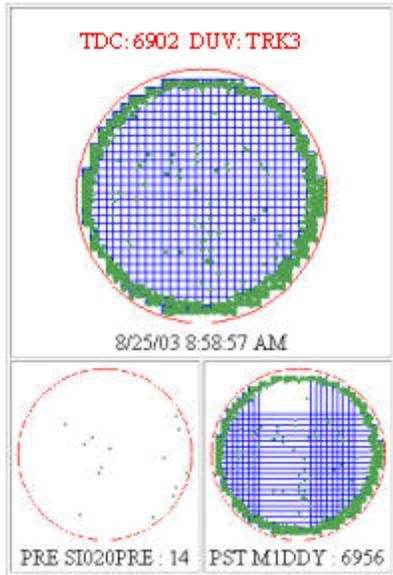
Fig.9: Micro-bubble defects
