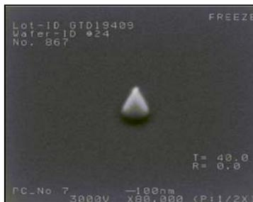
Figure 4: Typical cone defect.
