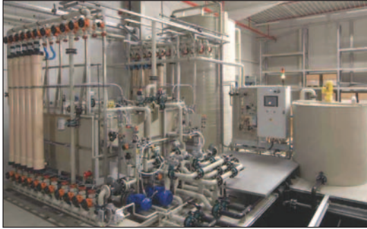
Fig. 2: Pall dynamic membrane system for 10 - 30 m 3 /hr / 44 - 132 gpm of spent sawing/grinding process water, 2 x 75% capacity for redundancy, with process water supply unit
