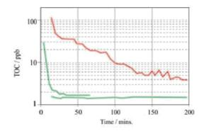
Figure 1. Downstream TOC levels during rinse-up for both an all-fluorocarbon filter (—) immediately after prewetting with 60/40 IPA/water, and a prewet all-fluorocarbon filter (—) using prewetting filter technology. The upstream TOC levels (---) are as shown.
