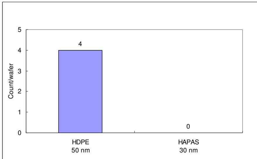
Figure 8. Filter comparison in killer defects on patterned wafer: Test fluid is non-PFOS TARC.
