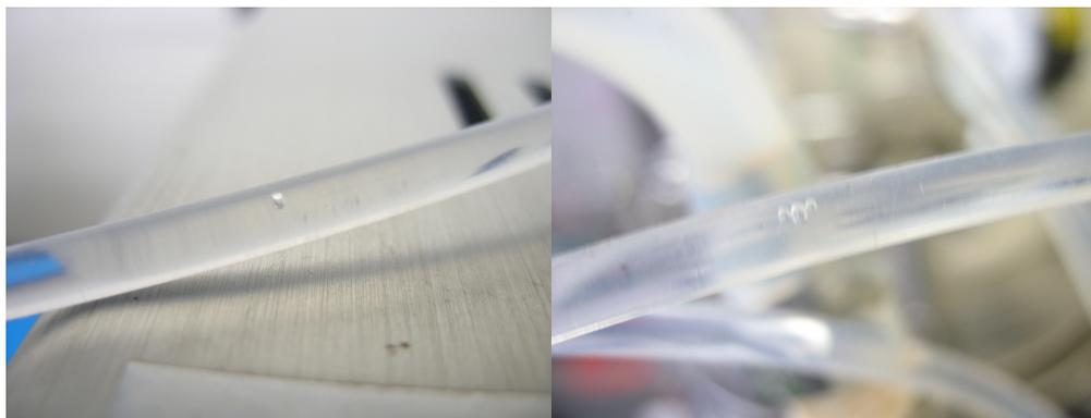
Figure 3. Visible bubbles found in the effluent of 30 nm HDPE filter.
