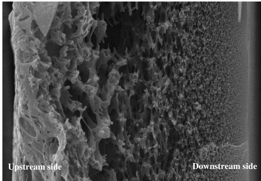
Figure 1. Cross-sectional SEM image of Highly Asymmetric Polyarylsulfone membrane.
