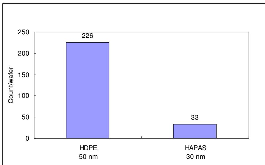
Figure 6. Filter comparison of defectivity on TARC-coated bare wafer: Test fluid is non-PFOS TARC.
