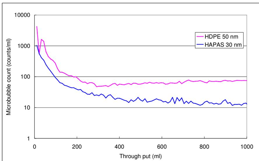
Figure 5. Microbubble count (>0.2  $\mu\text{m}$ ) in filter effluent of non-PFOS TARC.
