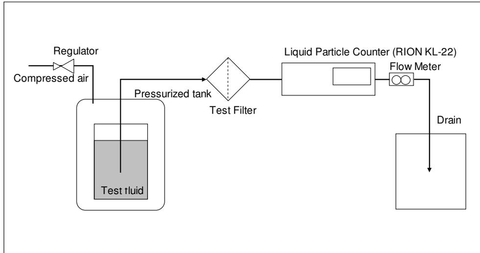
Figure 4. Experimental apparatus for microbubble measurement in laboratory testing.
