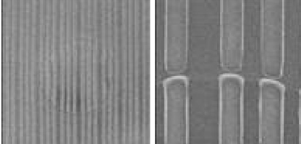
Figure 7. SEM images of a killer defect: Left, whole view; Right, enlarged view at the edge of the defect.
