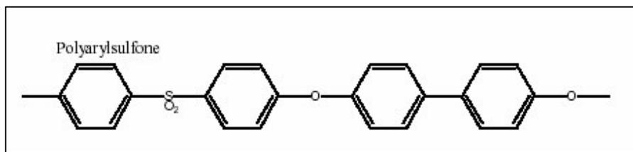
Figure 2. Bond-line structure of Polyarylsulfone.
