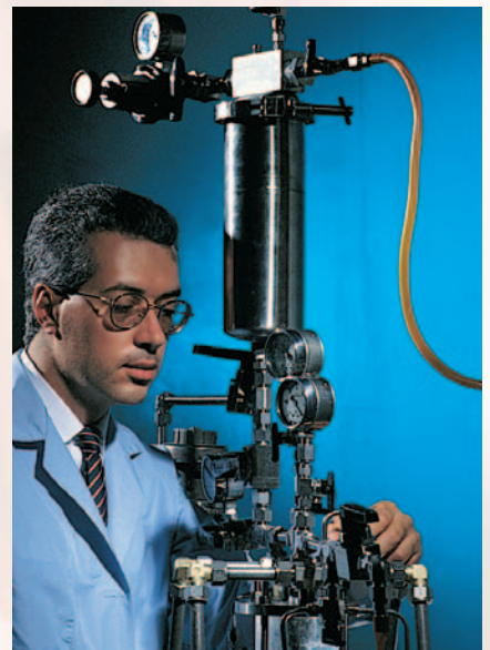
SLS prototype backwash test assembly
