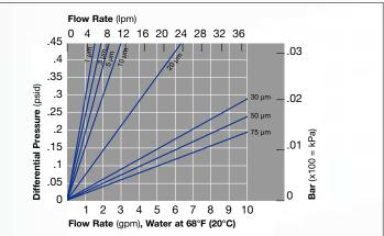
Flow rate is per 10" (25.4 cm) cartridge. For liquids other than water, multiply differential pressure by fluid viscosity (cps).
