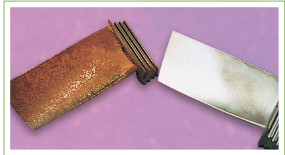
Left: Deposits form on a turbine blade.
