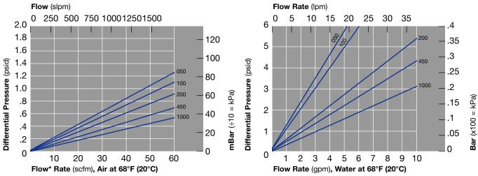
Flow rate is per 10" (25.4 cm) cartridge. For liquids other than water, multiply differential pressure by fluid viscosity (cps).
