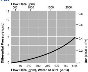
For liquids other than water, multiply differential pressure by specific gravity.
