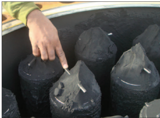
Figure 7: Coreless 1 um absolute graded pore depth filters after successful run of 20 months
