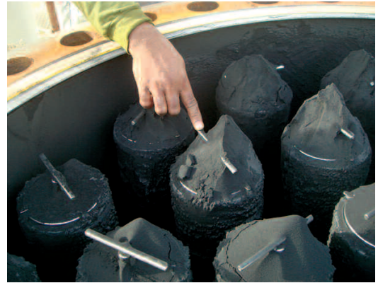
Pall's Coreless filters after a successful run of 20 months
