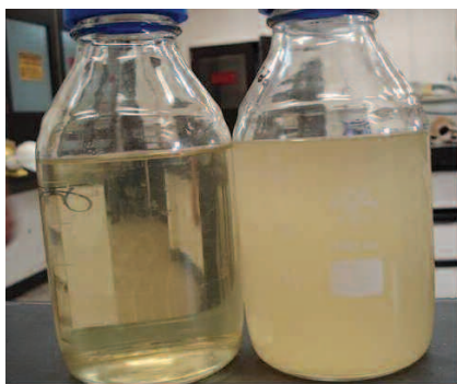
Condensate samples collected at Site C at the outlet (left) and inlet (right) of Pall's coalescer test unit
