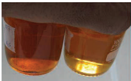
Condensate samples collected at Site B at the inlet (left) and outlet (right) of Pall's coalescer test unit
