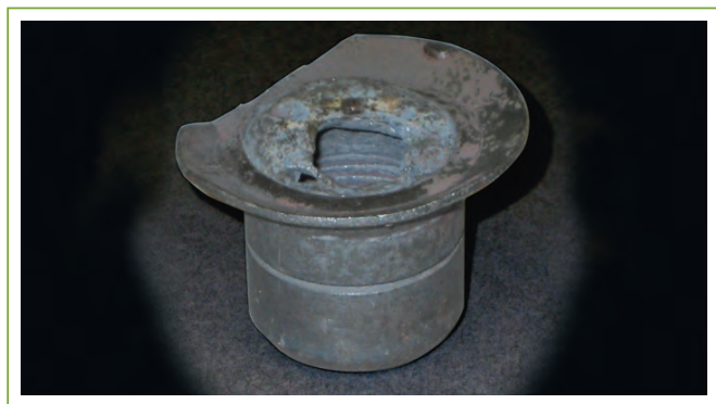
Damaged NOx burner tip due to contaminants
