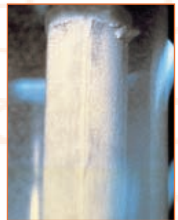
Element with permanent cake ready for resumption of forward flow.
