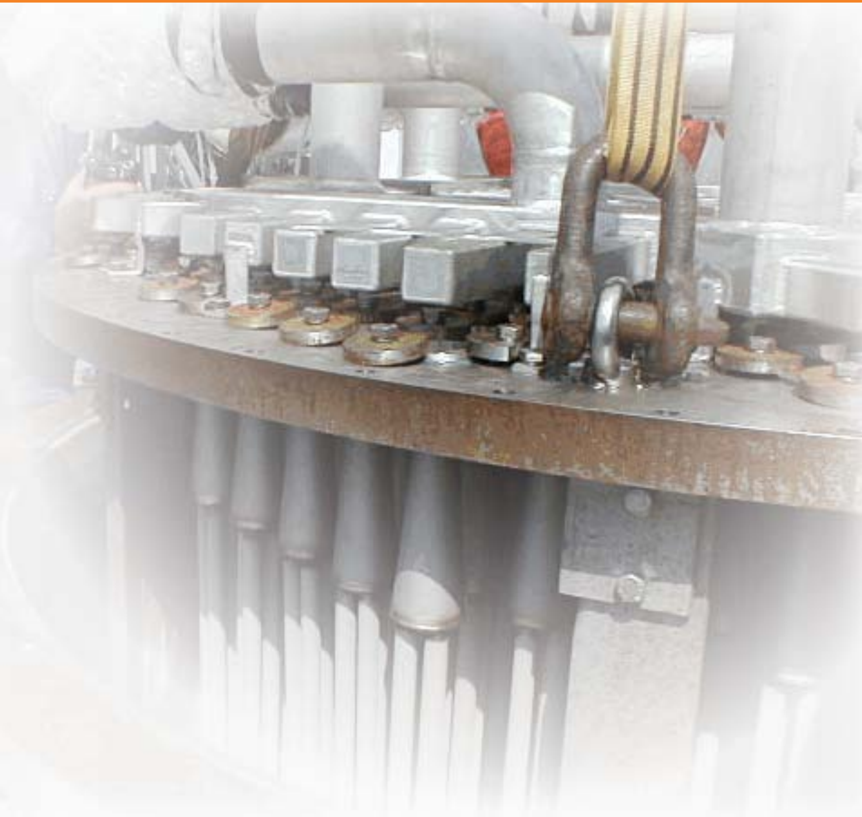
Pall jet pulse blowback system utilizing AccuSep® tubular filters. Filter tubesheet with filters being installed into the pressure vessel.
