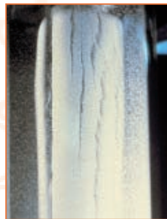
Reverse flow effectively dislodges nonpermanent cake.
