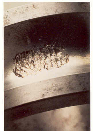
Typical bearing erosion caused by silting particles not removed in time.
